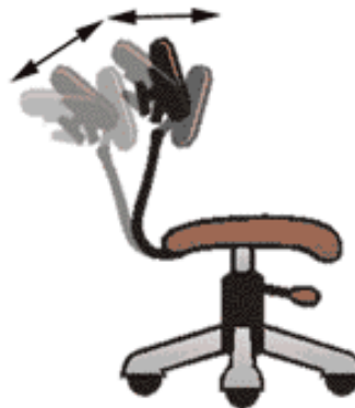
Figure 4: Adjust the position of the backrest so you can sit back in the chair, without the front of the cushion pinching the backs of your knees.
