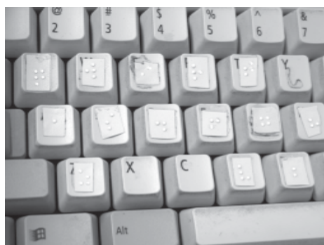
Figure 19: Learners helped the teacher make Braille letter labels and stuck them on the correct keys
